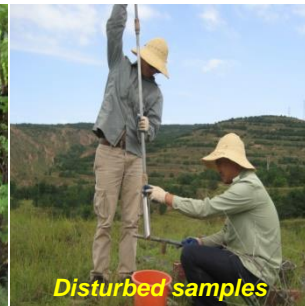
Soil moisture measurement
