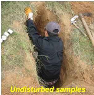
Soil moisture measurement
